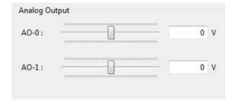
The output voltage for each of the devices analog outputs can be set here. Either move the slider to the required level or if you need to set an exact value, write the voltage value directly to the input text boxes. The value is than set when pressing enter or the input field looses its focus.
