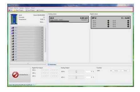
The main view of CeboLab is split into two parts. The upper part, highlighted in red, is always visible. It is not directly bound to a specific device, but some functionality (e.g. Project) works with the active device.
