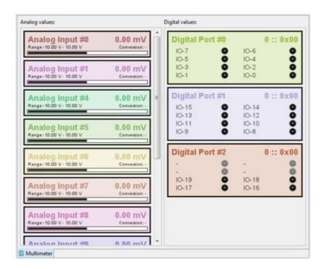
The analog display is very self-explanatory. Left is the name of the input and on the right, the active voltage is displayed. The **Range** on the left shows the active input range. If value conversion is used, the range is fixed as well. In this case, the active conversion is shown next to **Conversion**. The bar at the bottom of each input shows the position of the current value inside the current range.
