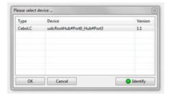
What follows is the device selector on the left. It lists all candidates for an update. Select the device to update and continue by clicking **OK**. If you have connected more than one device, use the **Identify** button. Clicking on this button turns off the identify LED for 500 ms.
